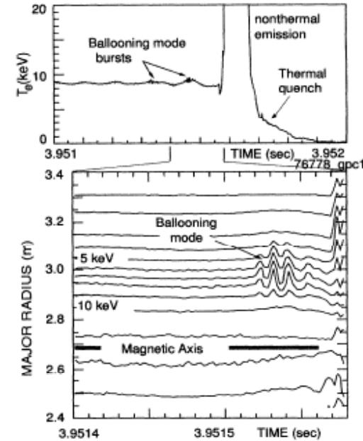
FIG. 7. The experimental ECE signals.
