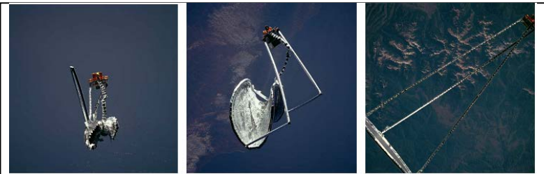
Fig. 1 Spartan 207 衛星での IAE (Inflatable Antenna Experiment) の展開挙動 (Photo Credit: NASA)
